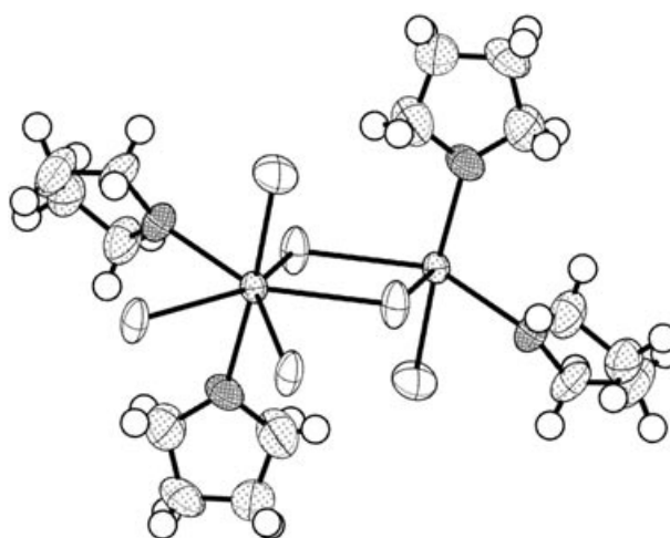
Figure 2. X-ray structure of the linear polymer [CeCl(μ-Cl) 2 (THF) 2 ] n .
